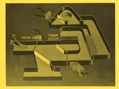
Here we see the mode door in the *heat* position, allowing air to come out the heater outlets. The power servo is keeping the temperature door in a position that allows just enough hot air from the heater to mix with cold air from the evaporator to keep the in-car temperature at 73 degrees.
