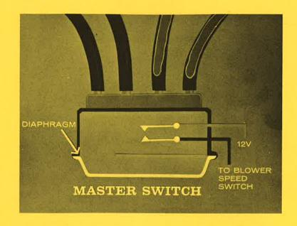
Here it is. The master switch. The master switch turns the blower "off" and "on", and also directs vacuum to the outside door recirculation diaphragm. Notice that a visual inspection of the diaphragm on the master switch will tell you if vacuum is applied, the diaphragm will be collapsed. If not, it will be expanded.
