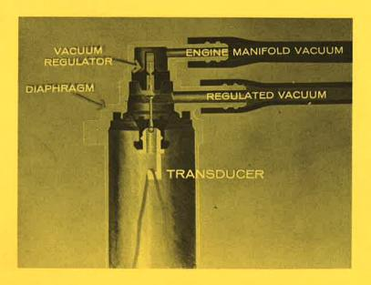
The increased voltage to the transducer heats the wire and relaxes the tension, which reduces the regulated vacuum.
