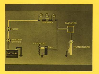
Let's move the dial to maximum cooling—that's 65 degrees— and see what happens. Rotating the dial increases the signal voltage to the amplifier. The amplifier then increases the voltage to the transducer.
