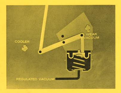
A strong vacuum at the power servo means "make it warmer", while a weak vacuum means "make it cooler."
