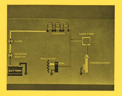
The amplifier output voltage may range all the way from zero volts in cold weather up to nine volts in hot weather. This amplified variable voltage is directed to the transducer to interpret the variable voltage from the amplifier and translate it into regulated vacuum.
