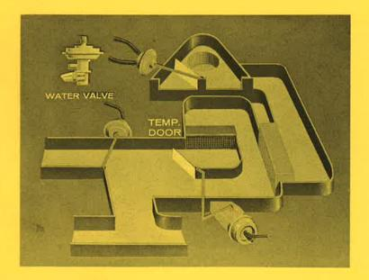
Reduced regulated vacuum to the power servo permits the servo spring to move the linkage which moves the temperature door to the maximum cooling position. This also moves the blower-speed switch to the high-speed position and causes the vacuum valve to supply full vacuum to the water valve, cutting off water flow to the heater core.
