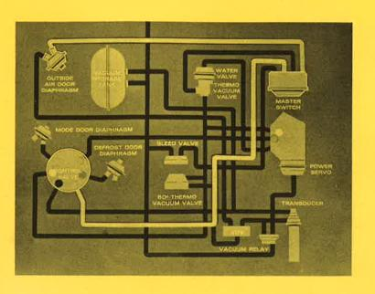
The master switch is a vacuum-operated electric switch. It is operated by vacuum directed to it from the vacuum valve on the control panel. Moving the sliding lever on the control panel to "off" cuts off vacuum to the master switch. This turns off the blower, and, because the same vacuum that is operating the master switch is also directed through the switch to the outside air door, the door closes by spring force when the vacuum supply is cut off.
