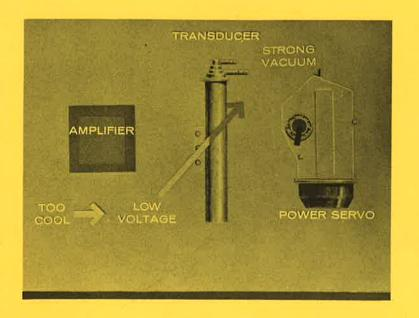
If the "sensors" signal it is too cool, a low voltage causes a strong vacuum, making it warmer. With this sensitive electronic-vacuum system in complete control, any temperature changes are counteracted as soon as they occur and the temperature is stabilized within one degree.
