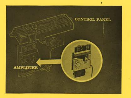
In the control panel — along with the rheostat operated by the dial — is a transistorized amplifier. This amplifier magnifies the small voltage variations caused by changes in temperature at the "sensors". Even a change as small as a tenth of a volt can be built up enough to shift the system all the way from heating to cooling.
