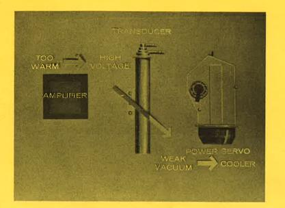
If the "sensors" signal it is too warm, a high voltage causes a weak vacuum, making it cooler. Now then, we are well on our way toward learning how the system operates.
