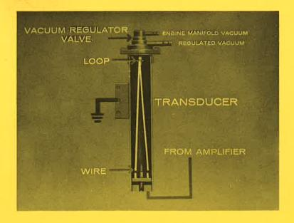
As you can see, the wire from the amplifier is connected to the wire inside the transducer. The wire inside the transducer is looped over the bottom of the vacuum regulator valve and down to a ground connection. For this reason, the transducer must always be grounded. The amplifier voltage goes through this stretched wire and heats it, causing it to relax some of its tension. Variation in amplifier voltage causes a variation in tension on the wire.
