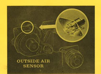
Next, we have the outside-air "sensor." It is the weather forecaster for the system. The outside-air "sensor" is located in the outside air-inlet duct where it can check the temperature of all incoming air and alert the system as to whether heating or cooling will be required.
