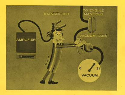
The amplifier-output voltage and full engine vacuum are supplied to the transducer. It must interpret the amplifier voltage and operate a needle valve to regulate vacuum so that it can be used to operate the Comfortron system. Now, let's take a closer look and see how the transducer works.
