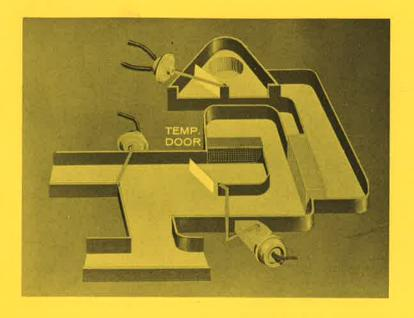
The linkage is connected to the temperature door. The power servo can assume any number of positions, because it is supplied with regulated vacuum. But, moving the temperature door isn't the only job it performs.
