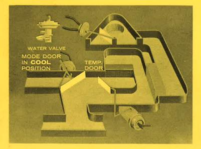
Rotation of the vacuum valve also cuts off vacuum to the mode door and the spring moves it to the air-conditioning mode so that the cold air will be directed to the air-conditioning duct and out the nozzles. Now, let's look at another very important part of the system.
