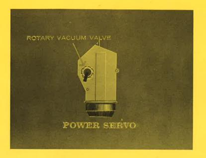
The power-servo linkage also operates a rotary vacuum valve to operate the mode door which was formerly called the selector door. This door directs air out the heater outlets or air-conditioning outlets. The power-servo assembly also operates the water valve and the blower-speed switch which controls blower speed automatically.
