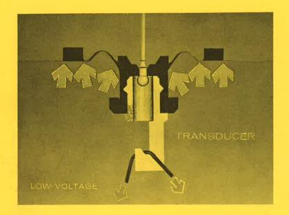
The diaphragm is balanced between atmospheric pressure and the tension on the wire. When the voltage is low, the wire tightens up and pulls on the diaphragm, producing a strong vacuum. When the voltage is high, the wire relaxes, producing a weak vacuum.
