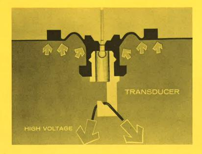
Let's take a closer look at the vacuum regulator, because for diagnosis purposes it is important for you to remember the lower the voltage, the higher the vacuum—and the higher the voltage, the lower the vacuum.
