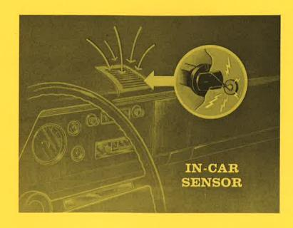
The in-car "sensor" is mounted so that the sunshine warms it just as it does the driver. It casts the deciding vote by signaling the amplifier that cooler air is required even before the driver is aware of the change. If a lower or higher in-car temperature is desired, rotation of the dial is all that is required.
