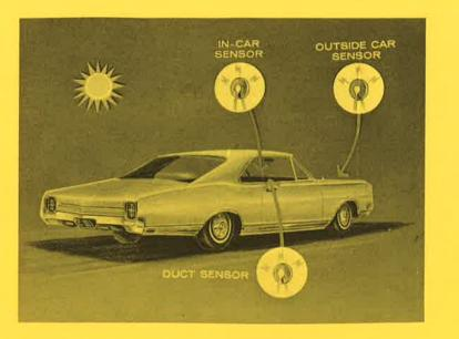
Now, the early-morning sun slowly raises the outside temperature and the outside "sensor" detects this increase. It signals the amplifier to compensate for the warmer air entering the cowl inlet. The duct "sensor", constantly checking the tempered air in the duct, also signals the amplifier. The combined signal to the amplifier from these two "sensors" then is averaged, leaving the big decision to be made by the in-car "sensor".
